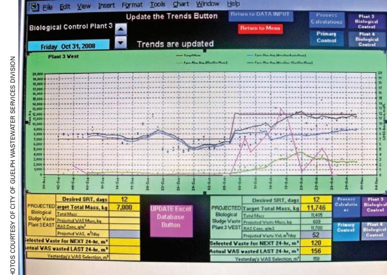
Data obtained from process centrifuges are entered into a data management and trending program.
